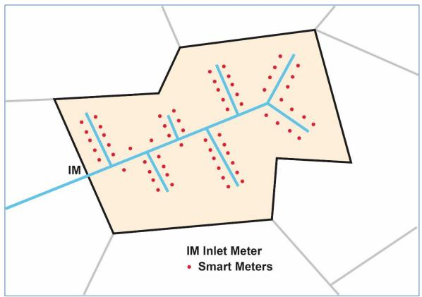
**Figure 3:** The principle of a DMA. The entire distribution network is divided into 22 independent and transparent DMA's. An Inlet Meter measures the volume of water delivered to the DMA, and the sum of the readouts from the Smart Meters represents in comparison the billed volume inside the area.
