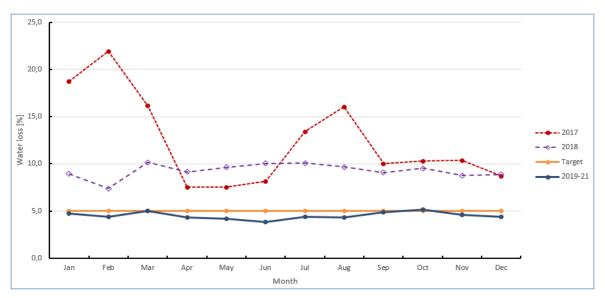
Figure 2: Monthly average water losses at BWC in from 2017 to 2021. The Water Loss is calculated as Potable Water Volume input from Utility Treatment Works subtracted Billed Metered Consumption.
