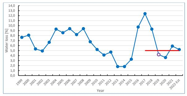
**Figure 1**: Yearly average water losses at BWC from 1999 to 2021. Water loss is calculated as Potable Water Volume input from Utility Treatment Works subtracted Billed Metered Consumption.
