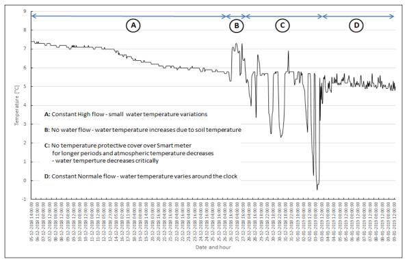
Figure 7: Example of temperature readouts from Smart Meter during different operational conditions.
