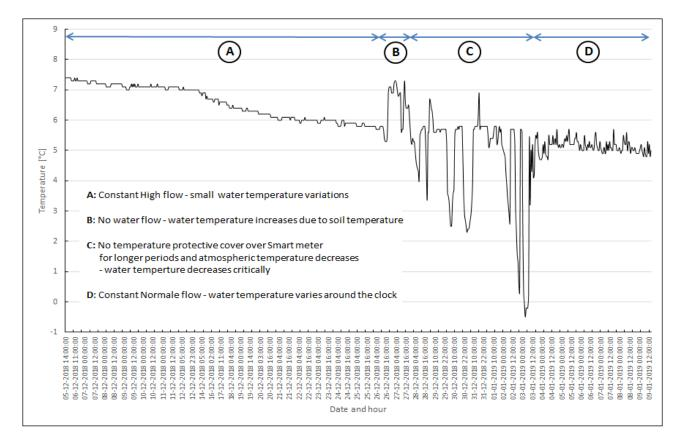
Example of temperature readouts from Smart Meter during different operational conditions.
